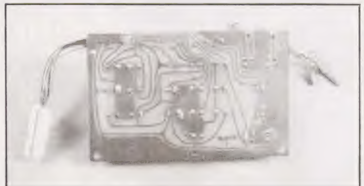
The keyboard PCB foil layout. Don't let the solder get bridged!
